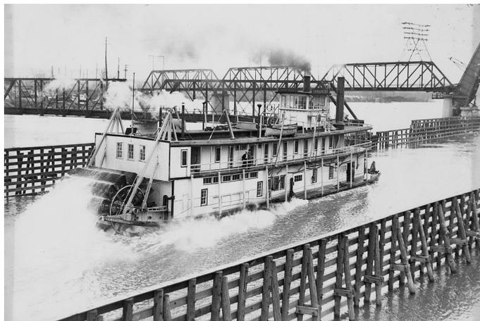
**COMANCHE (To478)**, a USE towboat for the Illinois River was also built by DBBCo in 1915 and carried 340-hp G&E engines, although their dimensions are not given in Way's Steam Towboat Directory. Her pitman appears to be constructed with a steel lattice design.
