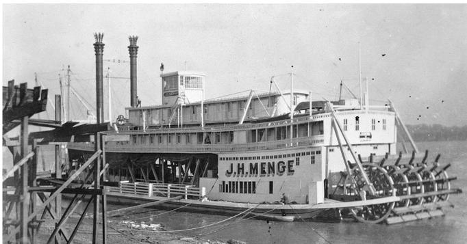
*J. H. MENGE (2844) was a 1910 Howard-built cotton packet with G&E compound engines 13's, 26's - 8 ft. stroke. A brief bio of J. H. Menge appears in the March 2014 REFLECTOR.*
