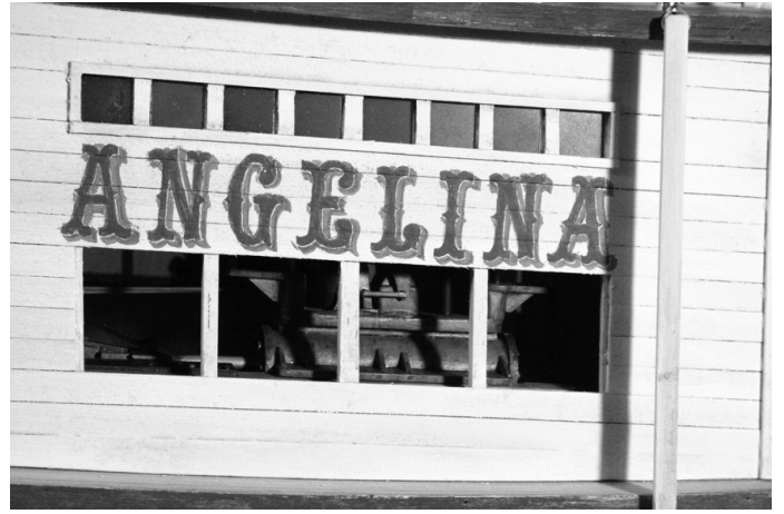
Starboard engine cylinder can be seen through open vents.
