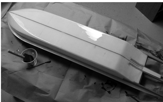
Finished and fiber-glassed hull.
