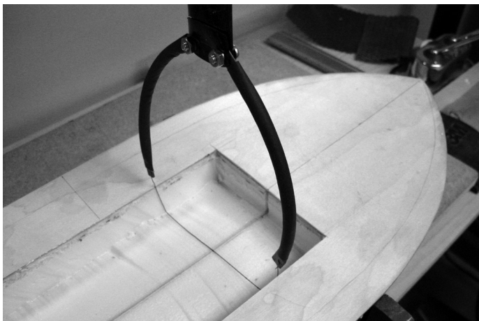
Hollowing out the “equipment well” with a hot wire cutter.
