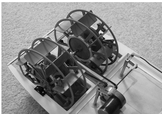
Motor and drive belt set-up. Photos courtesy of John Fryant.
