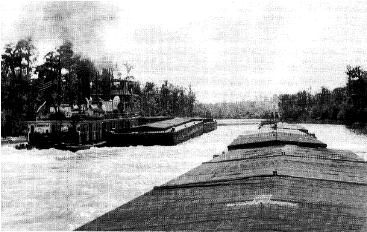
THE INTRACOASTAL WATERWAY TRAVERSED SWAMPS FOR SOME 30 MILES BETWEEN THE EAST ENTRANCE AT MISSISSIPPI SOUND TO THE INNER HARBOR LOCK AT NEW ORLEANS. HERE, THE CORDOVA (T0510), TWIN-PROP, 800 HP. STEAMER OF THE WARRIOR DIVISION, FEDERAL BARGE LINES PASSES BY WITH EASE ABOUT TEN MILES FROM NEW ORLEANS
