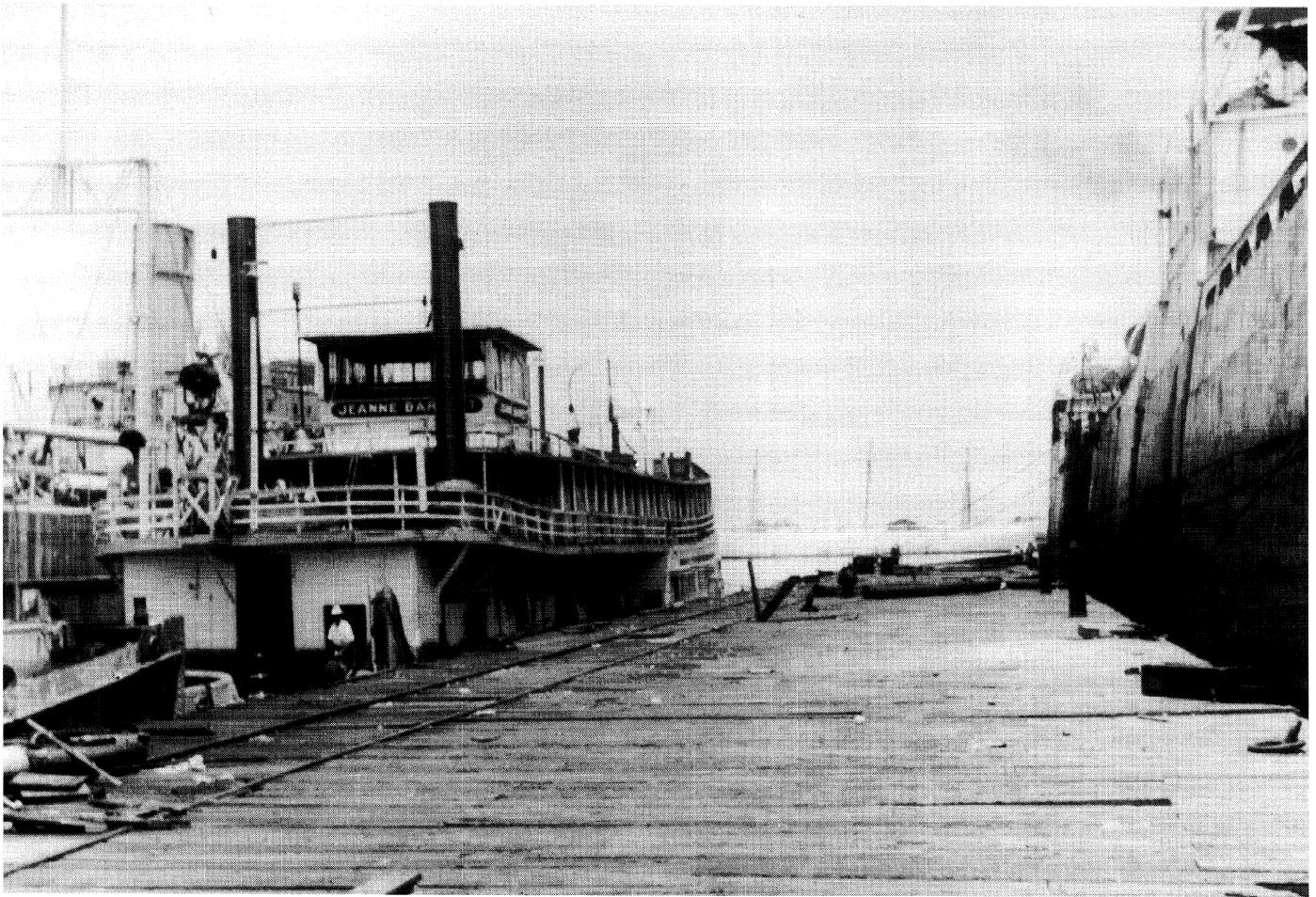
THE JEANNE BARRETT (T1350) WAS A WELCOME SIGHT AMONG THE LIBERTY SHIPS AND TANKERS WHICH FILLED THE SLIPS AND CROWDED THE ANCHORAGE IN UPPER MOBILE HARBOR. JEANNE BARRETT WAS BUILT AT PADUCAH AS THE WHITE SPOT (T2637) IN 1915, 112.7x26x2.9, ENGINES 13'S-6 FT. STROKE FROM THE PACKET CITY OF PEORIA AND RENAMED BY THE BARRETT LINE ABOUT 1927. WATCHMAN HOWARD CLEVELAND WELCOMED THE OUT-OF-PLACE OHIO RIVER YAWL.
