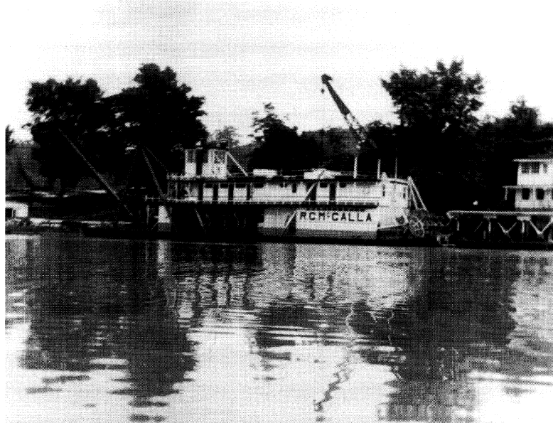
Above, the laidup BALDWIN with two boilers, fore and aft in the hold, Gillett & Eaton engines. Below, snagboat R. C. McCALLA, steel hull.
