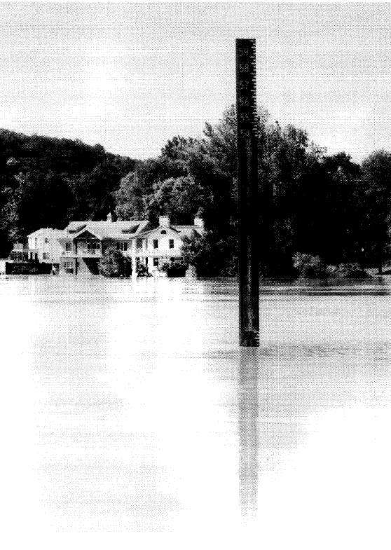
Noon, Sept. 18, 2004. The river gauge at the Army Corps of Engineers Repair Station at the junction of the Muskingum and Ohio Rivers stood at 41.0 ft. The top of the gauge, for reference, is 60 ft. Fred Rutter Photo
