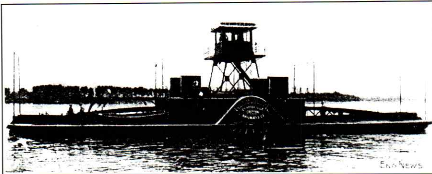
FIG. 1. GASOLINE CAR-TRANSFER BOAT ON THE OHIO RIVER; FOR THE INTERURBAN CARS OF THE EVANSVILLE RAILWAYS CO., EVANSVILLE, IND. (Evansville, Henderson & Owensboro Division.)
