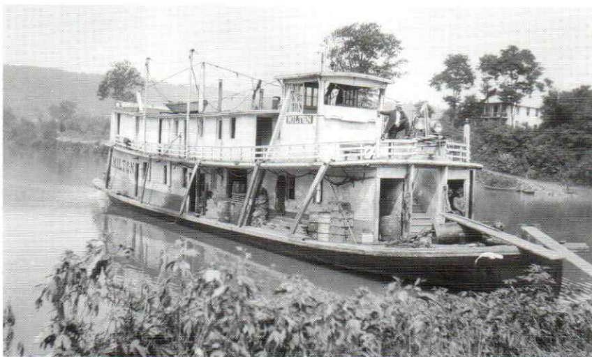
The boiler deck guard on the MILTON did not match that on the QUEEN CITY but carried out the packetboat design; no rockers, however. On the Little Kanawha River, the guards were cut down to fit in the 125x22 foot lock chambers in five dams providing slackwater to Creston, WV. Photo by W. S. Pollock, August 1920.
