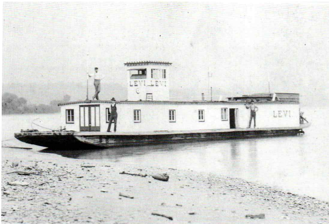
The LEVI ready for service in the Madison trade, 1890. We estimate her measurements about 40ft.x10ft. That must be designer Edward Turner standing proudly by the jackstaff; the more mature Jim Reed below. Air cooling for the mules is available by opening the double doors.
