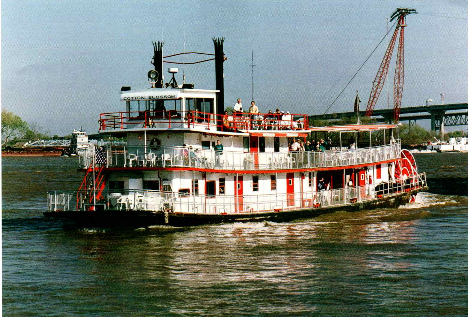
COTTON BLOSSOM built by Ward, Charleston, WV, 1928, 135x28, 275 hp. Caterpillar diesel, passenger capacity 349.
