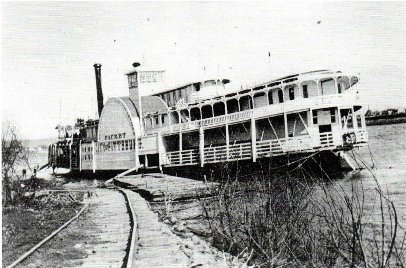
The CITY OF PITTSBURG (1122) at the Knox Boatyard on the Harmar side of Marietta in early spring 1899. She appears complete, ready to go but because of a mixup in ordering boilers she has missed her scheduled trip to the Mardi Gras, - finally left Pittsburgh March 28. The Scotch Marine boilers were unsatisfactory and replaced a year later. The boat burned April 20, 1902 with 81 lives lost.
