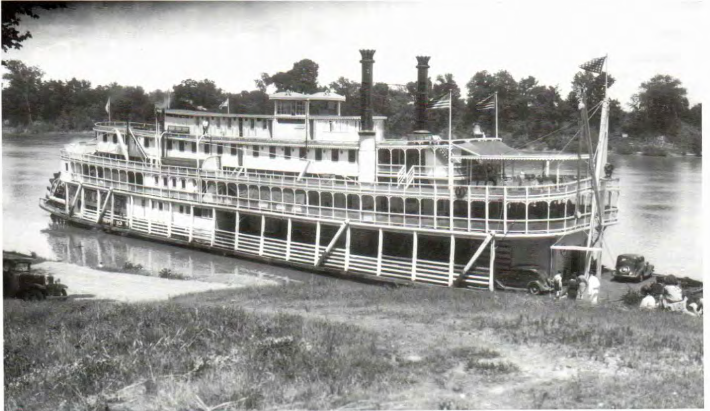
The GORDON C. GREENE before and after the 1937 replacement of the crew texas. Above, with the old texas divided by the pilothouse, raised just 28" in 1936 when the passenger texas was built. Print, J. Sutphin.
