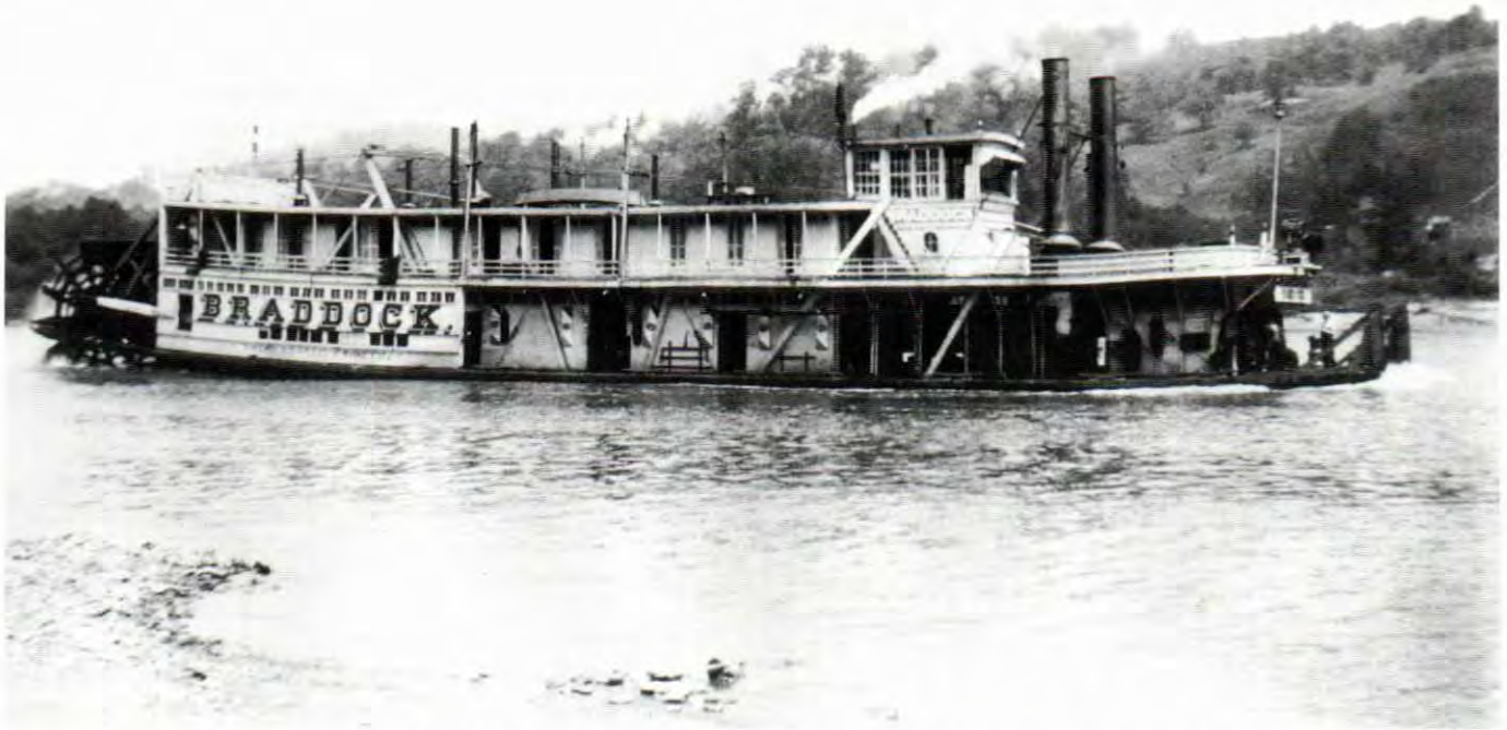
This is the first BRADDOCK (T0290), one of the poolboats on which Jake Yonker fired the boilers. She was built in 1900 at Elizabeth, Pennsylvania, 135x24x4 and owned by the American Steel & Wire Co. She had pop, instead of lever, safety valves but engineers could get around these, too. Photo Murphy Library, LaCrosse.
