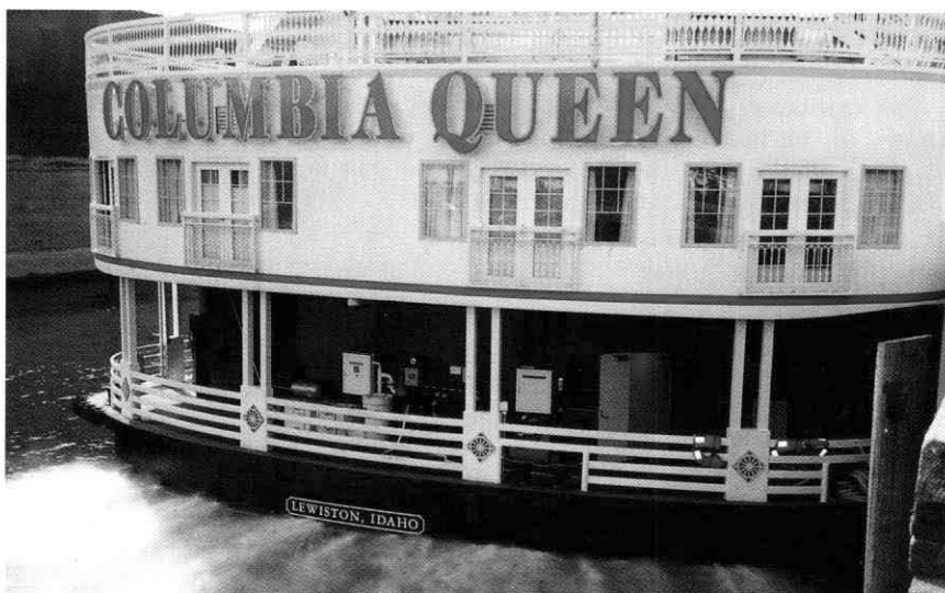
This view of the stern shows the spray system which absorbs the noxious exhaust fumes from the diesel engines. Don Chalmers.
