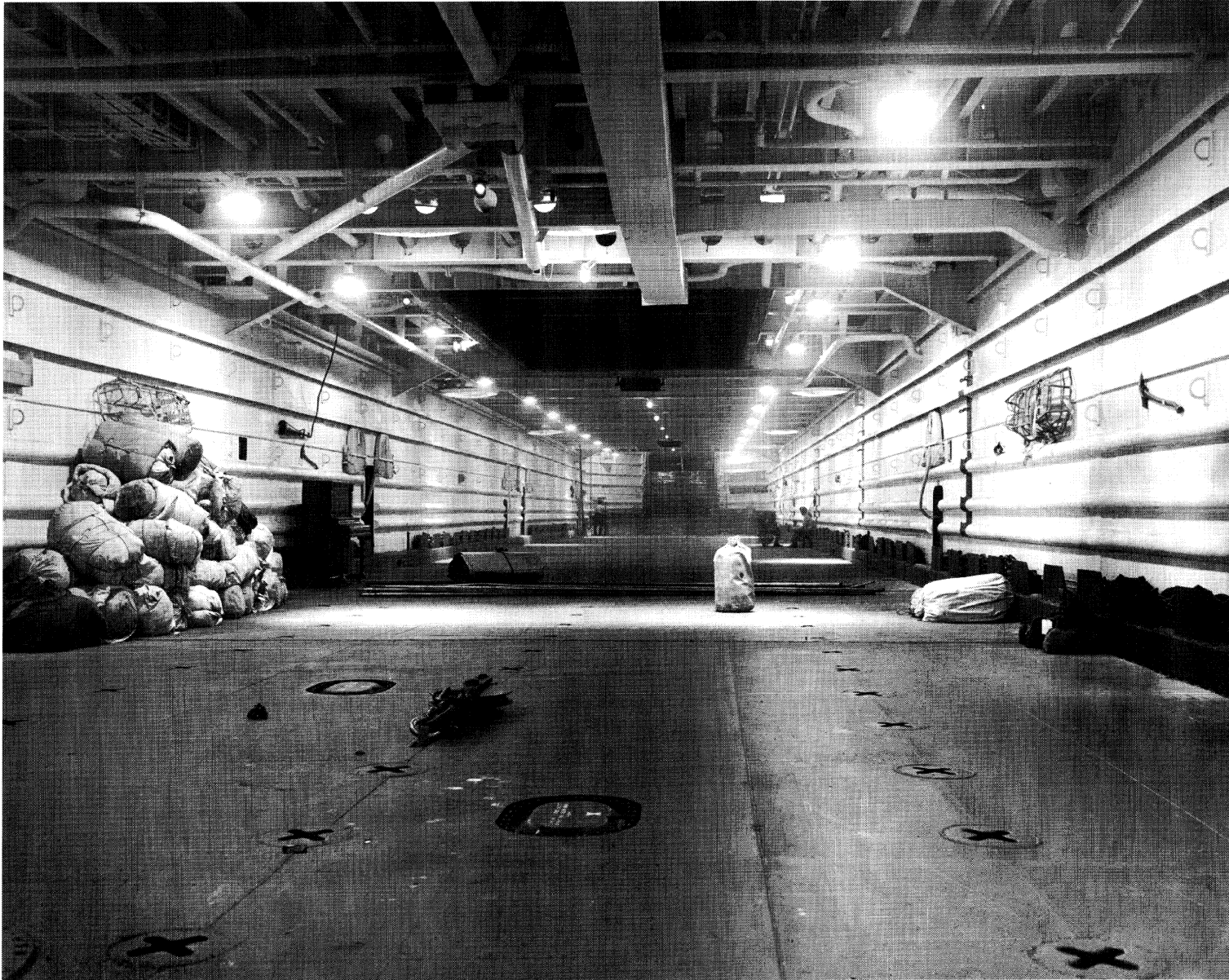
NO. 4 This is the tank deck of an LST and we guess it is looking toward the bow judging from the curved bulkhead at the far end. Six-by-six trucks piled high could be accommodated along with jeeps, trailers, artillery, tanks and a variety of tracked vehicles.
