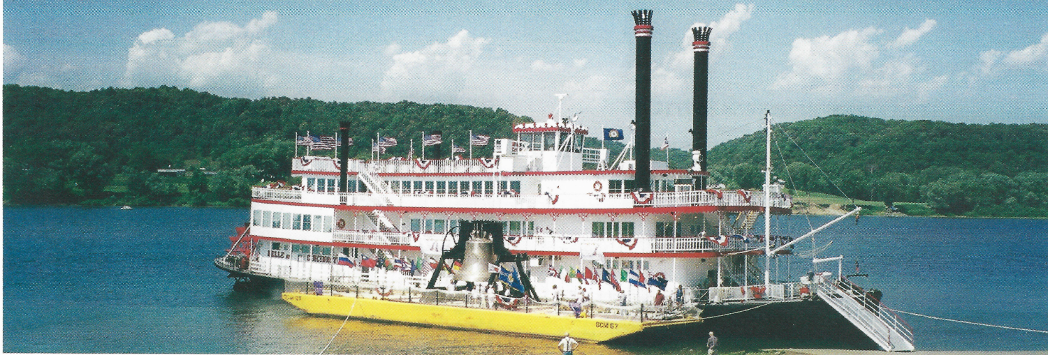
BELLE OF CINCINNATI with the Peace Bell at Carrollton, Kentucky. Propulsion by sternwheel with twin screws in reserve; three diesels total 2,010 horsepower. Photo by Gayle Hindman.
