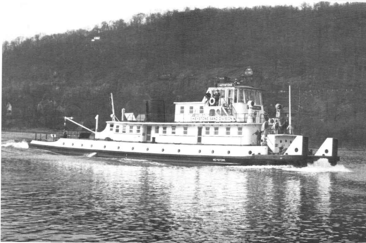
The towboat design with quarters for the crew down in the hull and a row of portholes was first offered by Dravo in 1940 with the twins DUCTILLITE and SEMET-SOLVAY. The design was lengthened ten feet to 145x27x12 for the KEYSTONE built in 1945 pictured here. The 760hp. served well for the sand trade but was hardly adequate for the fifteen and twenty barge tows of Union Barge Line, - but Clare liked her.
