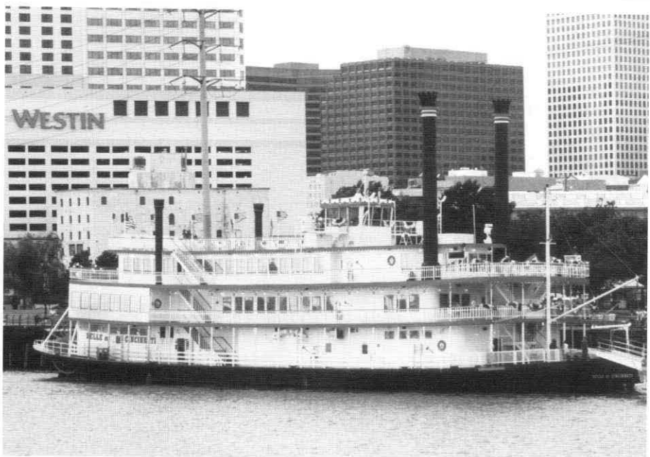
Once a tart but now she's a belle: The BELLE OF CINCINNATI at New Orleans before leaving with the barge carrying the 33 ton World Peace Bell. Built by Atlantic Marine, Inc., Jacksonville, FL in 1991 she is 201'x49.5'. Three diesel engines: Hydraulic drive to the paddlewheel plus twin props. Passengers, 1,000. Bill Judd photo.
