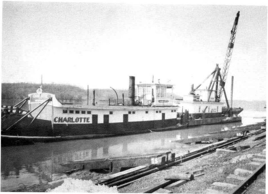
The CHARLOTTE towed the new steel wharfboat down to Huntington from the Acme Boiler Works on April 9, 1931. This steel hulled boat was built for stock by Marietta Manufacturing Co. in 1927, 80.1x22.6x2.7. She worked under charter for the Corps of Engineers on the Missouri River in 1928 but did not find a buyer, perhaps because she had only 120 hp. She was sold to the Powhatan Mining Co. in 1950 and renamed CHIEF POWHATAN.
