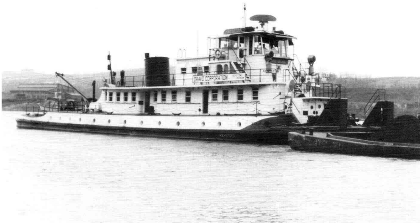
Capt. Clare Carpenter moved from relief master to regular master when Union Barge Line took over the MV. KEYSTONE from the Keystone Sand Division, Dravo Corporation in 1950. This boat was built in 1945 by Dravo, 145x27x11.9. The portholes gave light and ventilation to the lower level of the hull, a Dravo design trademark for several years, undoubtedly practical but at the time unusual and questioned by old-timers. Photo by William E. Reed.
