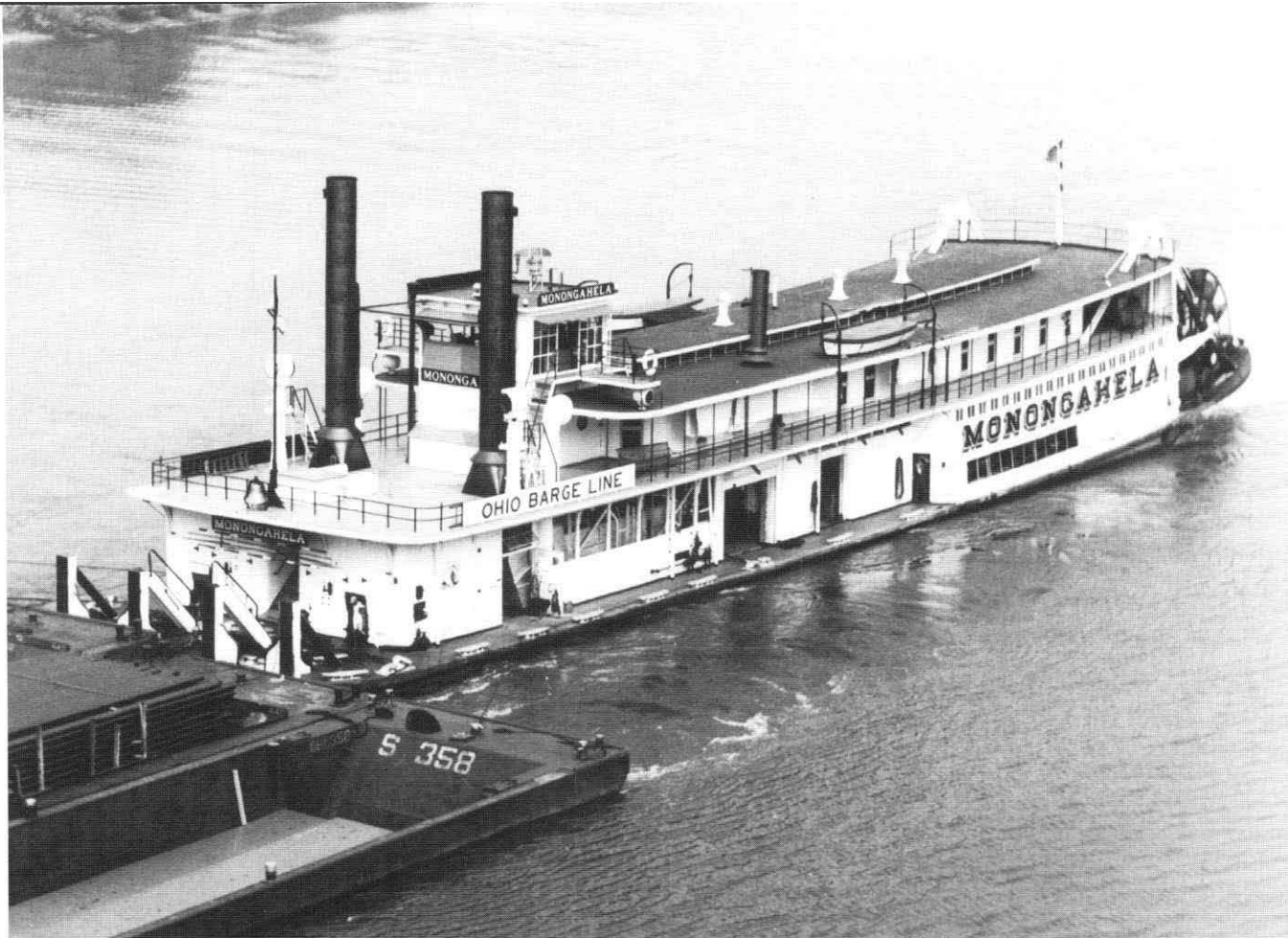
The MONONGAHELA (T1862) Built in 1927 at Ambridge and Coal Valley for Carnegie Steel Co. she was owned by Ohio Barge Line and under charter to Union Barge Line in 1943. 169.8x38.9x6.6, 18's,36's-8.6 ft. stroke, rated 1,400 hp. W. E. Reed photo from the Sewickley Bridge.
