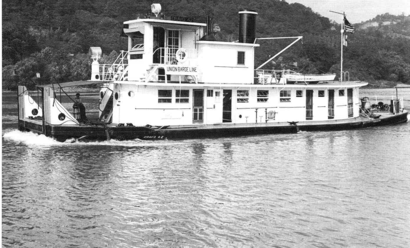
DRAVO 42 and her sister DRAVO 41 followed closely the design proven by the earlier PIONEER including the single screw in a Kort nozzle. 86.9x21.1x7.6 feet deep with a 350 hp Nelsco diesel engine.
