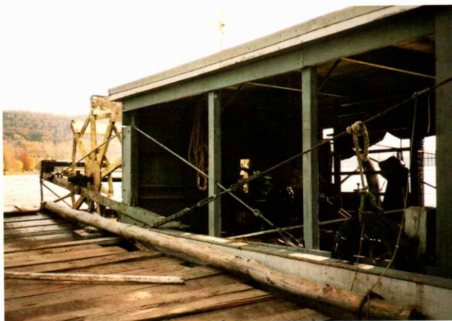
Engine room of the FALCON, sister boat of the ROARING BULL and with all the simple technology of a 1920s gasboat. Note the hog chains (cables) with turnbuckles to hold her in shape.
