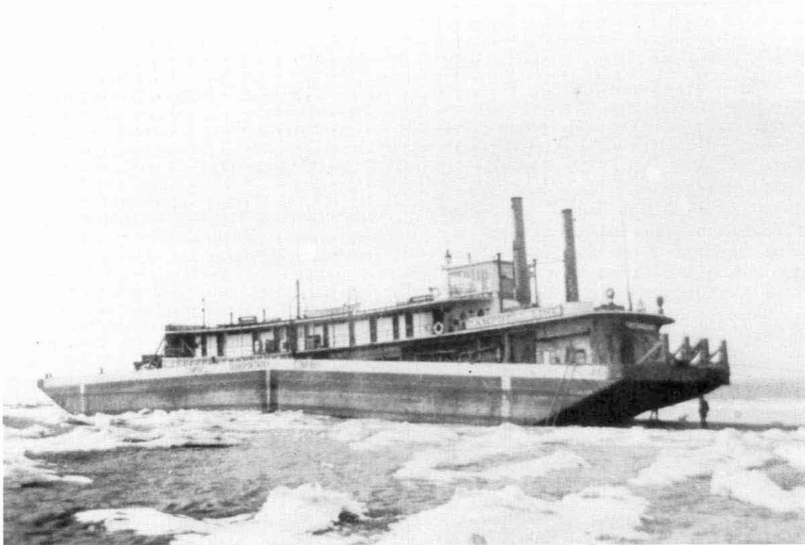
We found another view of the towboat ISTHMIAN (T1217) perched on the Wolf Island Bar, Mississippi River in 1935. The engineer thought to pump water into the barge for use in the boilers as the river fell. The unsupported barge broke as seen and the crew had a cold week until rescued. After repairs at Paducah, ISTHMIAN continued up the Ohio in January, 1936.
