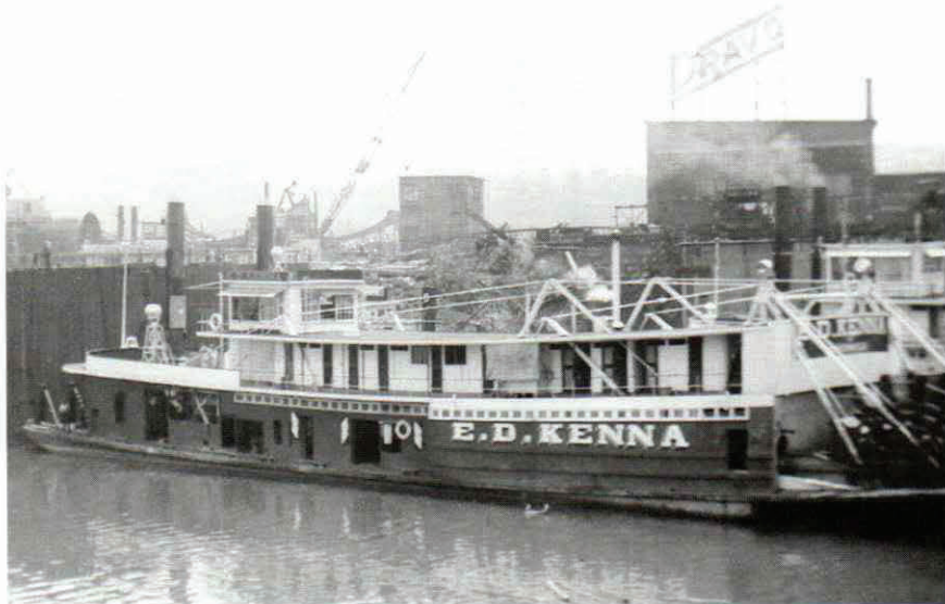
The E. D. KENNA (TO651) was less than two years old when Jesse was asked to stand pilot watch to Parkersburg in March, 1928. She was built by Wards, Charleston, WV for the Ohio River Co., 144x32.1x6.5, 700hp. Shown here at the Dravo marine ways, Neville Island, PA in 1936 where her length was increased by almost 30 ft. to 171.2 ft. J. Mack Gamble photo.
