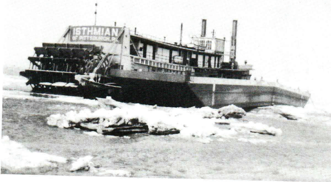
High, dry and cold on Wolf Island Bar, Mississippi River in December, 1935. The hump in the barge resulted from attempt to store boiler water.
