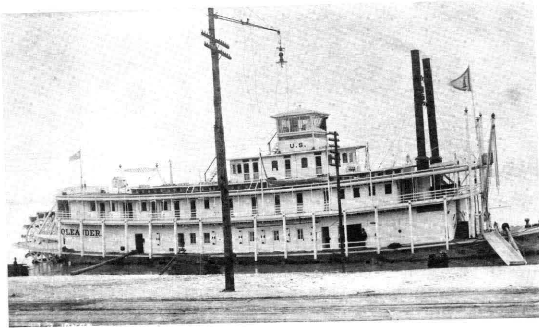
The Lighthouse Tender OLEANDER (4292) was built at Dubuque, Iowa in 1903 with a steel hull 165x34x7 in size. Readers of the Capt. Hoel story will recall that Supervisors enjoyed family vacations on board the Lighthouse Tender LILY so will not be surprised by the Tillman family sojourn of 1909.
