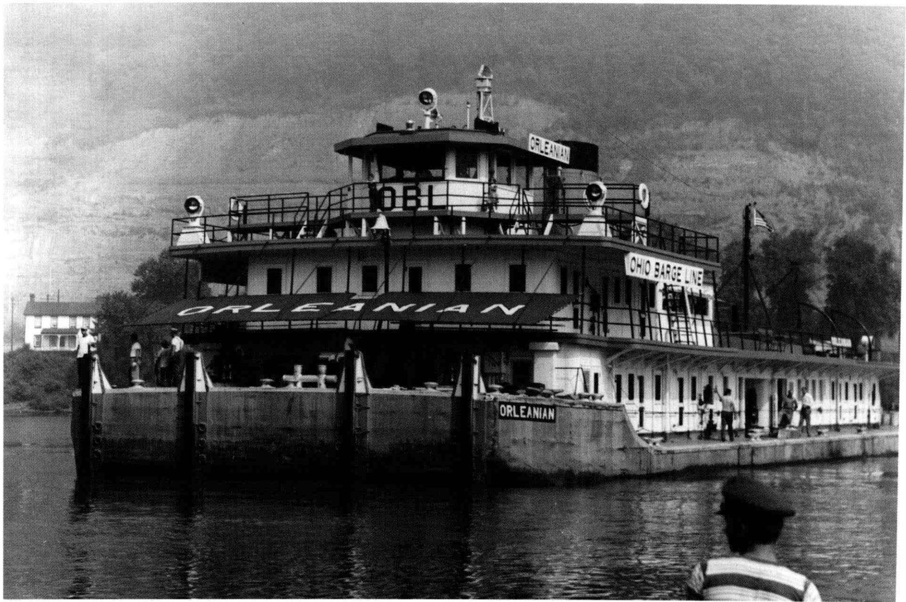
The Ohio Barge Line ORLEANIAN, originally the DPC BATAAN, is about to land at the Dravo Marine Ways, Neville Island on June 21, 1953. The high head incorporating the towing knees was a DPC feature.
