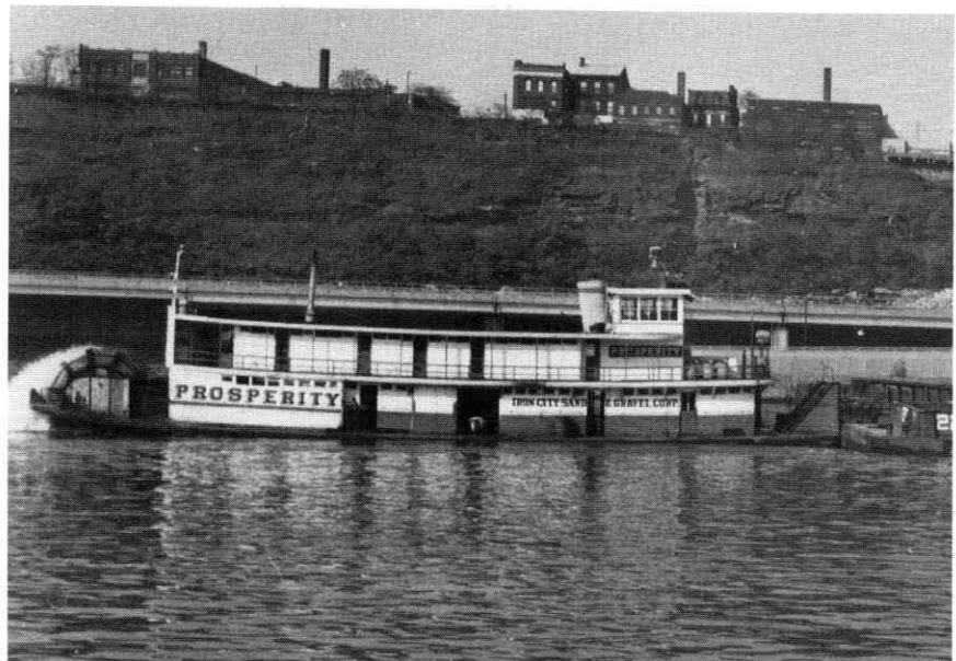
PROSPERITY after Iron City Sand & Gravel Corp. got her, now single stack behind the pilothouse and a 420 horsepower Superior diesel. Photo by Jim Swartzwelder.
