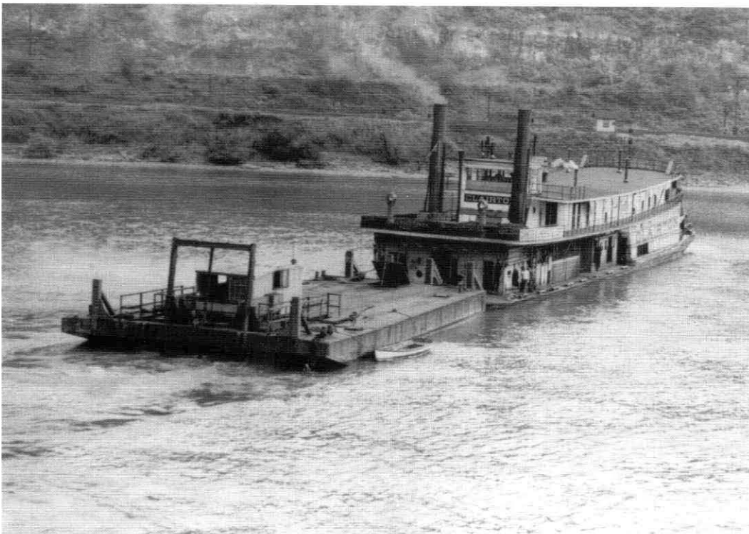
CLAIRTON (T0431) was built at Ambridge, PA by American Bridge Co. for Carnegie Steel Co. in 1919. The contraption ahead of the boat is a dynamometer barge; faced up to a dock the
