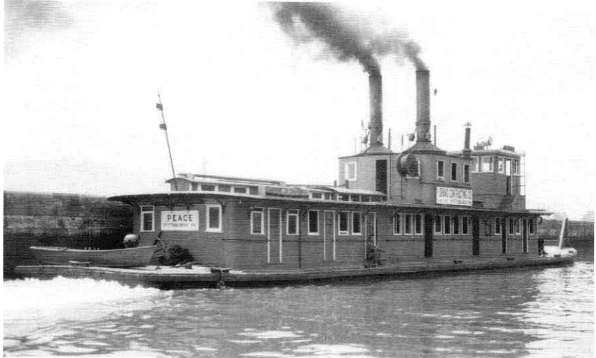
The PEACE (T2016) was not a new boat when Jesse noted her passing Catlettsburg in 1922 but she was still a novelty in towboat design. Built in 1917, 107.8x22x5.2, she was the Dravo answer to the prop designs of Ward Engineering beginning with the JAMES RUMSEY (T1337). W. S. Pollock photo.
