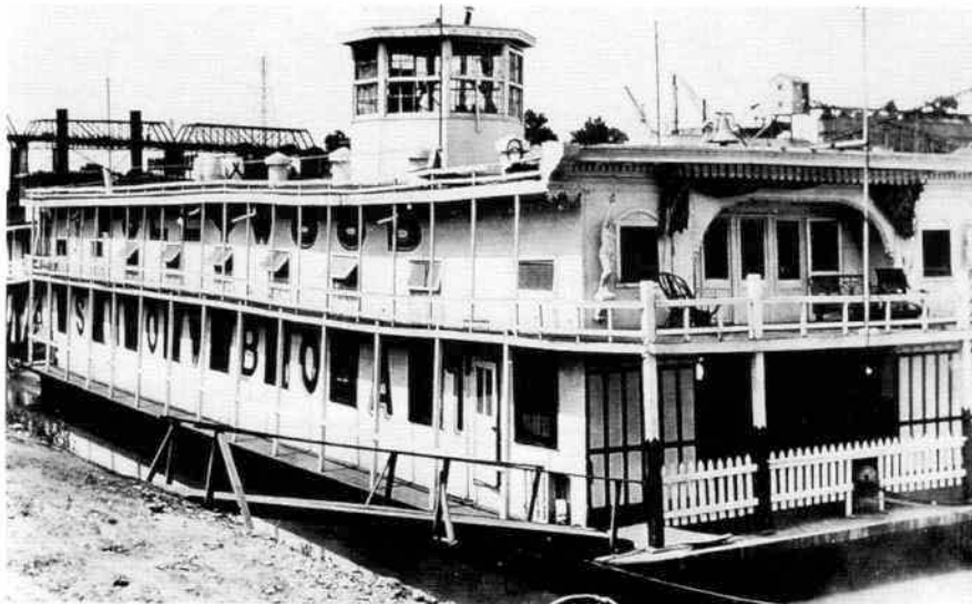
The HOLLYWOOD was rebuilt by the Menke brothers from the AMERICAN, later named COLUMBIA. She had a new hull 120x38 and noted for her fine interior and large calliope. Tiller lines lead from the octagonal pilot house back to the towboat. Photo could be at Nashville where the HOLLYWOOD had a long run in 1931.
