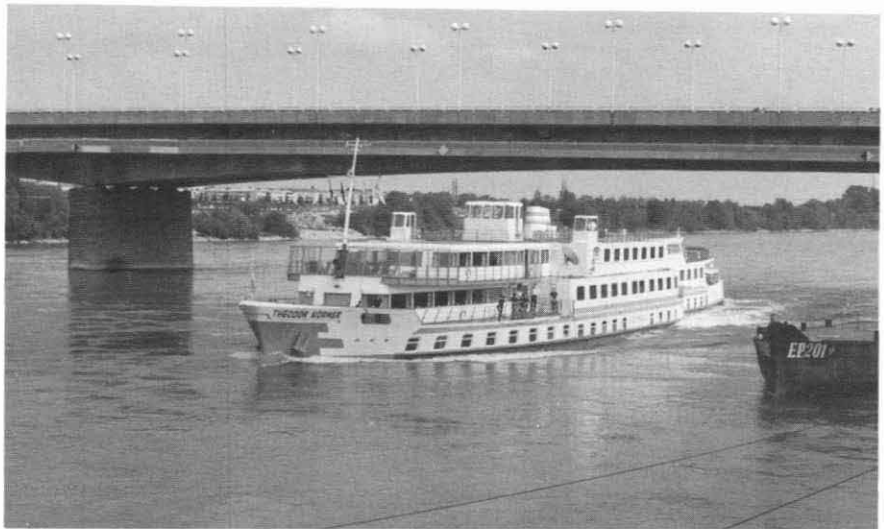
The THEODOR KORNER on the Danube River at Vienna, May 9, 1993. Owned by DDSG Line, the KORNER was built in 1965 and utilizes cycloidal, side propellers. The lowest windows forward are the diningroom with staterooms on the upper decks aft.
