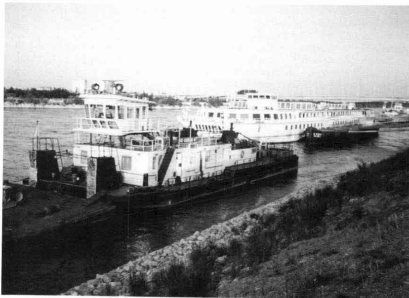
U.S. style push towing on the Danube dates from 1961. Above, a typical small towboat with lowering pilot house tied up at Vienna. One of the large, newer cruise boats is astern.
