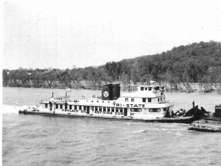
The mv. TRI-STATE of the Ashland Oil and Refining Co. fleet had the first installation of radar. When built at the Calumet Ship Yard & Dry Dock Co. in 1942 she was the last word in design and boasted two National Superior diesels, a total of 1,600 hp., twin prop. In size, the TRI-STATE was 145x31x8.8 ft.
