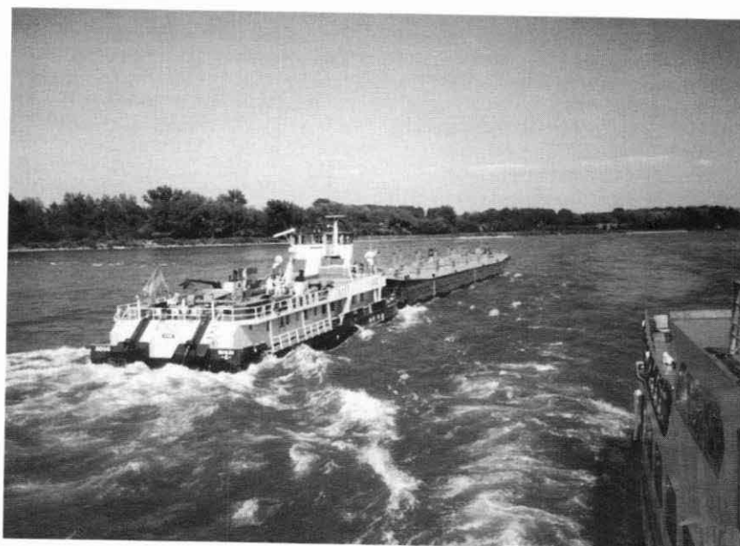
U.S. style push towing on the Danube dates from 1961. Above, a typical small towboat with lowering pilot house tied up at Vienna. One of the large, newer cruise boats is astern.
