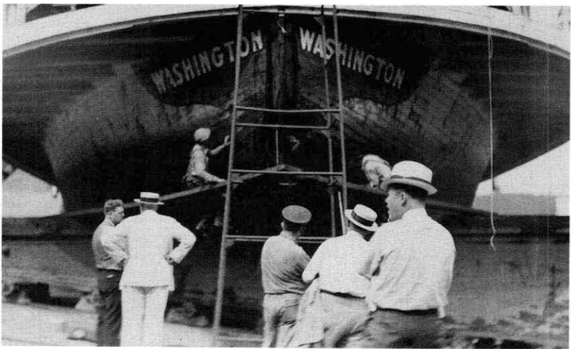
Two views of the damage to the WASHINGTON's bow after she was up on the ways at Dravo, Neville Island, PA. Wooden hulls were not in the Dravo line but repairs were completed in a week.
