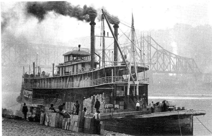
The S. L. ELAM at Pittsburgh on her first appearance after being bought by the new Liberty Line. She had been built in 1913 and had compound, non-condensing engines 12's, 24's-6 ft. stroke. She made one round trip Pittsburgh-Cincinnati with her cotton guards before going to the Mozena boatyard at Clarington for rebuilding as the GENERAL WOOD. Photo by Fred Way.
