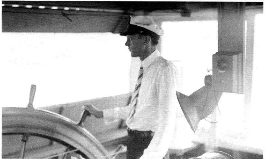
Capt. William S. Pollock on watch on the WASHINGTON, 1936. Note the sound tube from the engine room and the telephone to the right. Fred Way photo.
