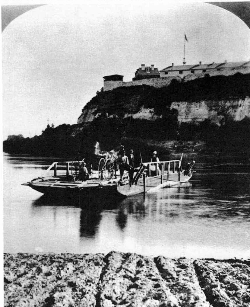
Constant current in the Mississippi supplied the power to get this ferry back and forth by use of cable and pulleys.. Fort Snelling appears on yonder hilltop.
