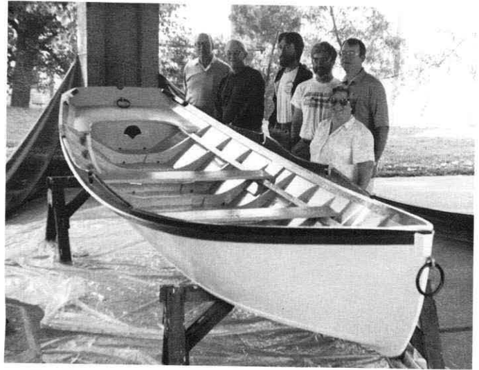
Six builders, six weeks and the skiff is completed. She is three inches wider because of the way the poplar sides bent around from stem to stern but otherwise closely matches the 1888 all oak original. The builders: J. W. Rutter, Jim Stephens, Doug Wallace, Paul Lewis, Nancy Riley and Bob Hill.
