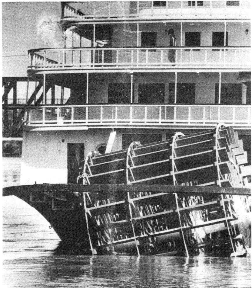
The last thing you expect to happen, does. The newly refurbished DELTA KING at Sacramento dropped her wheel in the river during mid-March when a weld let go. -Thanks to Hal Wilmunder for the newspaper picture.
