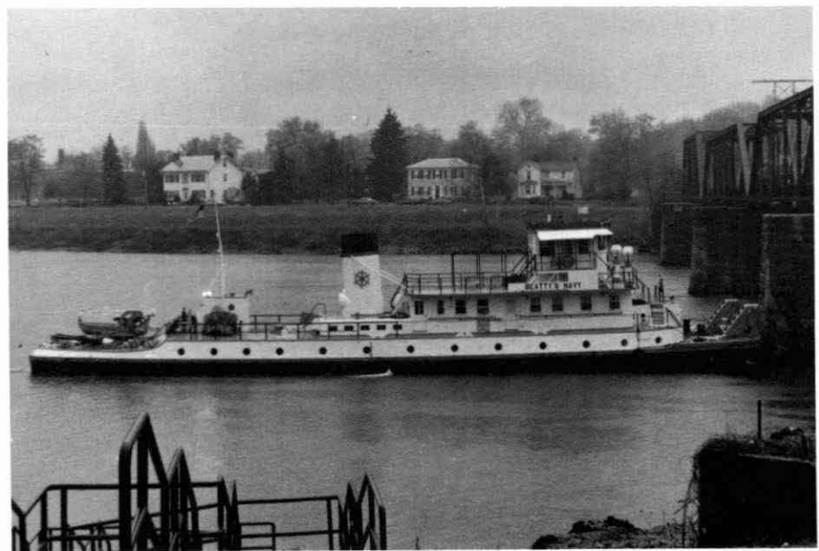
WAITING FOR THE RR. BRIDGE TO SWING OPEN, the 1800 hp., 135-ft. long CLARE E. BEATTY is in the Muskingum at Marietta to pick up the W. P. SNYDER JR.
