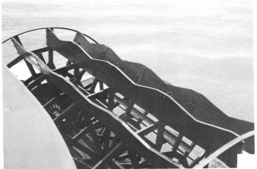
New paddlewheel design on the CREOLE QUEEN at New Orleans. Photographed April 18th by Judy Patsch. The excursion boat is pictured and described in our Dec. 83 issue, page 42. Judy neglected to say why the buckets, which are functional, were given a marcel wave.
