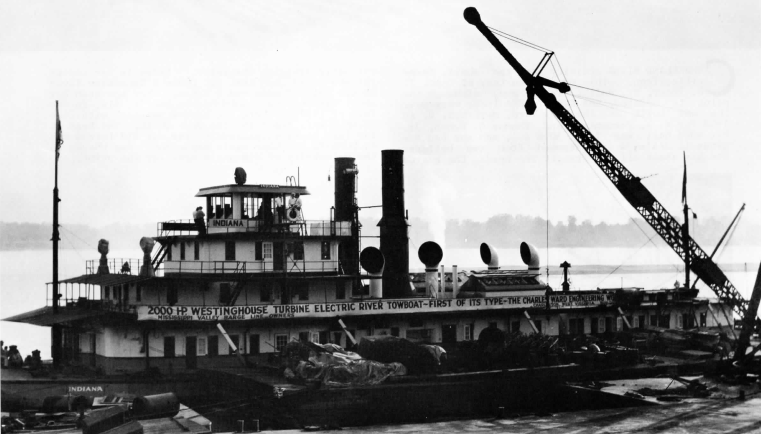
P HOTO taken by the U. S. Engineers, Memphis, in 1930 of the Mississippi Valley Barge Line's new towboat INDIANA. The long banner on the boiler deck rail reads: 2000 HP. WESTINGHOUSE TURBINE ELECTRIC RIVER TOWBOAT---FIRST OF ITS TYPE---THE CHARLES WARD ENGINEERING WORKS, CHARLESTON,
