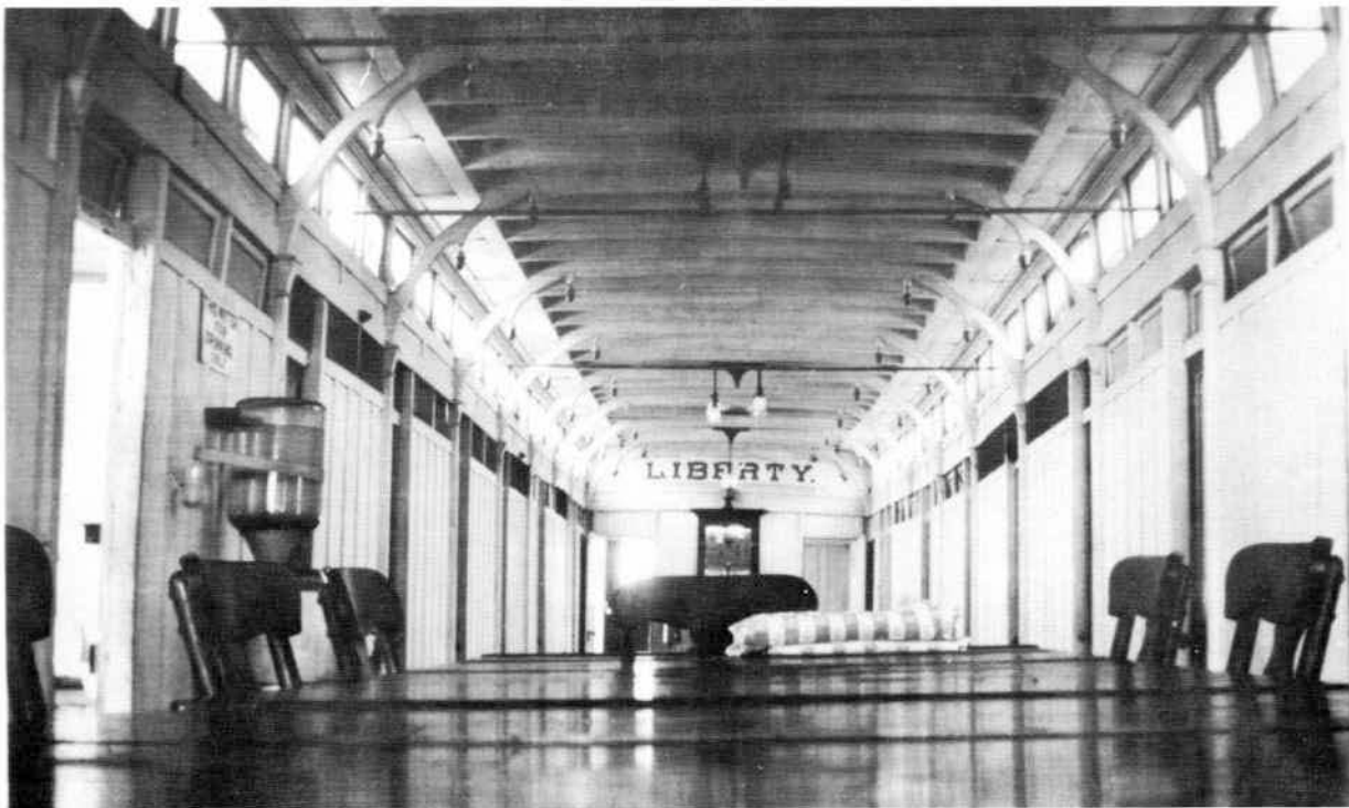
Looking aft in the LIBERTY's cabin after the rear staterooms were added. Cabin was 12 feet wide and from roof to
