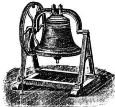
Ranging from 100 pounds to 350 pounds, mounted with IMPROVED PATENTED ROTARY HANGINGS, by means of which the Bell can be readily turned in the yoke, so as to present a new point for the stroke of the clapper. Frame of ash timber, iron stands, clapper springs, and iron wheel.
