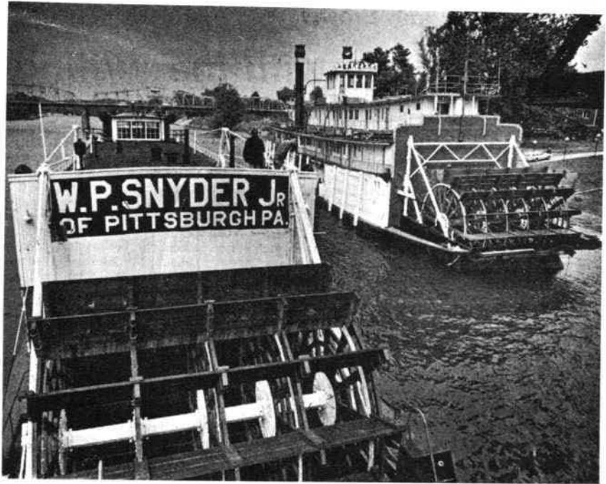
The W. P. SNYDER, JR. being maneuvered down the Muskingum in tow of the RICHARD NEALE and with the DIANNE NEALE as bow boat. The BECKY THATCHER, ex-MISSISSIPPI, now a restaurant boat, is off to the right. The SNYDER's stacks were lowered to clear the Putnam Street bridge. She was backed all the way out of the Muskingum.
