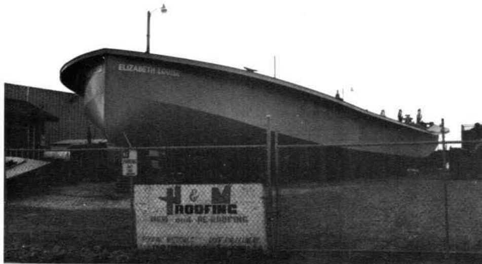
Steamer ELIZABETH LOUISE ready at the building yard for her 27-mile overland haul to the Sacramento River. The graceful proportions of her ½" steel hull are apparent here. She has 27 inches of longitudinal sheer. Read article at the left.
