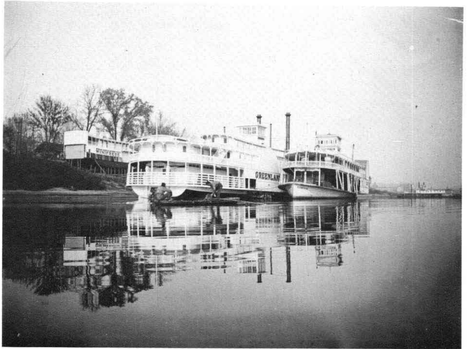
JESSE HUGHES took this early November 1903 picture when the GREENLAND was about ready for trials. It shows to some degree the peculiar "sternwheel" stern of the hull. The ZANETTA is riding light, now shorn of boilers, engines and paddlewheels; several years later the hull was used for the Kanawha River packet J. Q. DICKINSON. At left, on the stocks, is the towboat WINIFREDE under construction.
