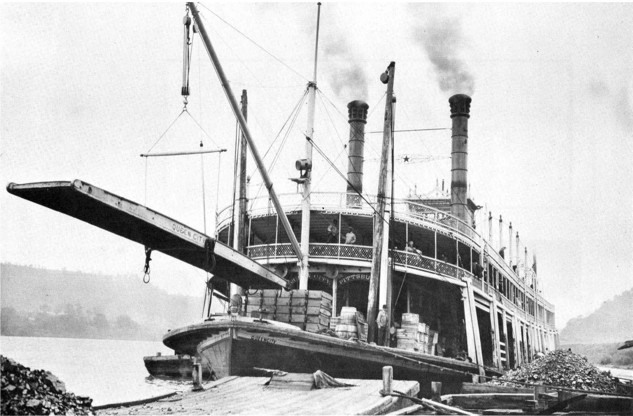
Taking on coal. These Pittsburgh-Cincinnati packets usually fueled at Ashland, Ky., Minersville (above Pomeroy), and Bellaire. We'd judge this is taken at the latter place. The coal was gravity-loaded from a tippel to a deck flat, then hand-shoveled aboard. She is downbound; see the hogshead and a tierce of straw-packed pottery from East Liverpool on the forecastle.
