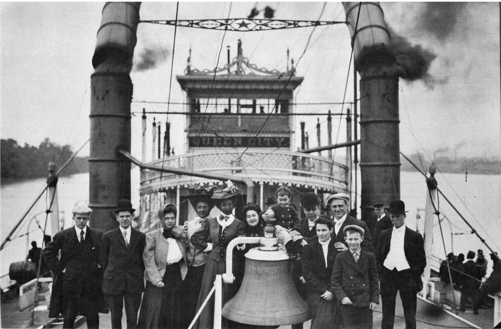
The roof bell long has been a favored place to take group pictures. Capt. J. Frank Ellison got this bell from the St. Louis Anchor Line. It had served on the side-wheel CITY OF ST. LOUIS. Today by a circuitous route it is on the DELTA QUEEN. The stacks are tipped back slightly in deference to a bridge. Deckhands await, extreme right and left, to wind the stacks back to the upright position.
