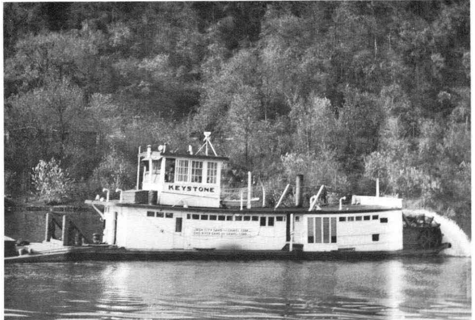
Diesel towboat KEYSTONE, picture furnished kindness of William E. Reed. Her pilothouse recently was moved from New Martinsville, West Va. to St. Louis (see story in left column). This wood hull sternwheeler was built at Pittsburgh in 1937 by Charles Zubik, 77.1 by 20. She came out with a Fairbanks Morse engine rated 180 hp. Iron City Sand & Gravel bought her from Zubik and later she long operated in the Ohio River Sand & Gravel fleet at New Martinsville. In 1952 she was given a new GM diesel, 240 hp. Last appeared in the 1960 edition of Inland River Record.
