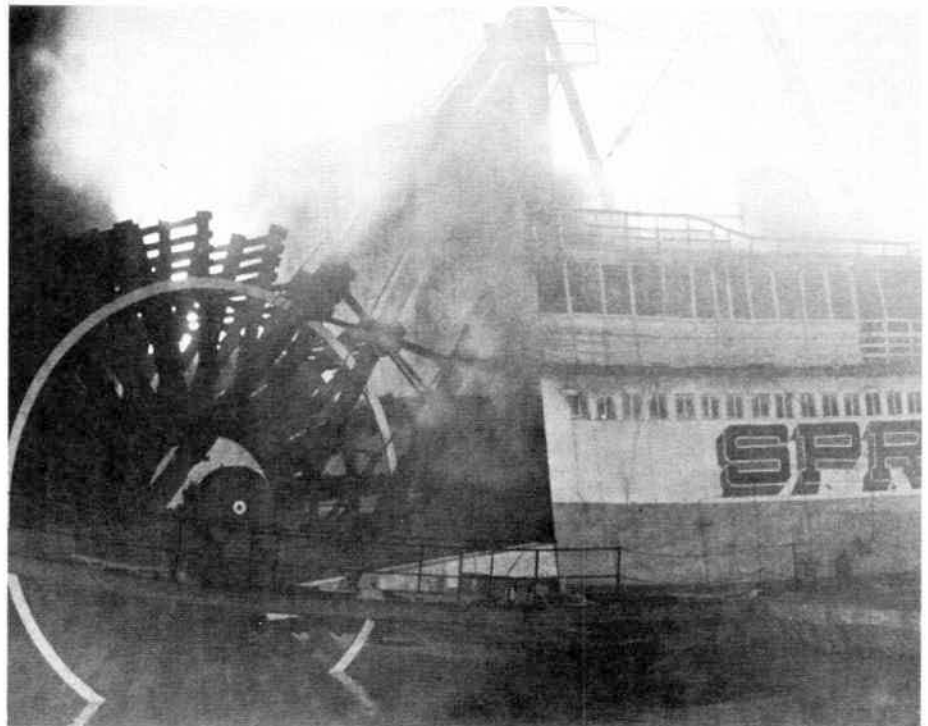
The blaze as seen by a photographer for the Vicksburg Evening Post. The morning after the night before the main deck didn't look too bad except for paint blistered from the steel bulkheads. Cabin and pilothouse were demolished and the stacks fell. She was afloat with the stern deep in the water (drawing maybe three feet more, aft) and the head away up looking at the moon. We would guess that the engine-room machinery, etc. was not badly damaged. Mississippi governor William L. (Bill) Waller visited the wrecked boat and pledged state support for rebuilding the SPRAGUE, and urged a nation-wide campaign for funds with $3 million as the tentative goal.
