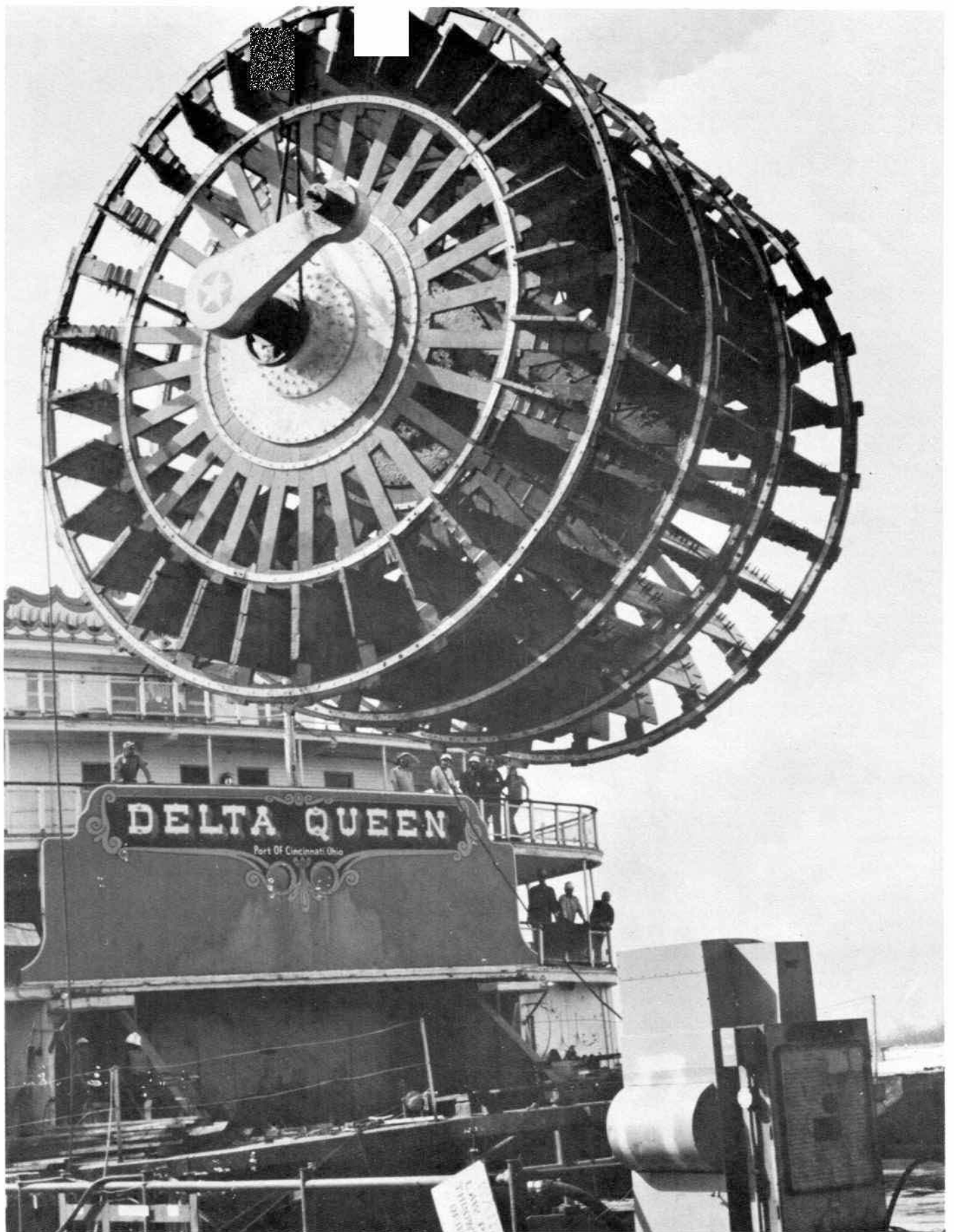
While Avondale had the DELTA QUEEN's wheel off this spring, they weighed it. Tipped the scales at 44 tons. -Photo from Delta Queen Steamboat Co.
