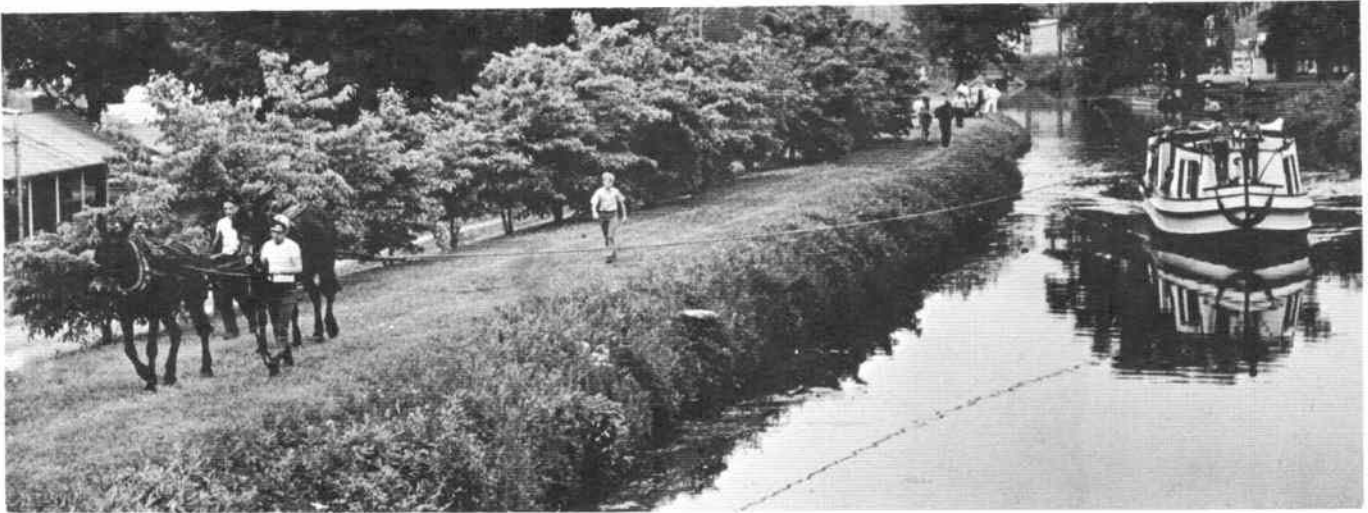
Along the towpath of the Ohio & Erie Canal at Canal Fulton, O., two mules in tandem pull the ST. HELENA II at a lively clip. Note that the tow line is not affixed to the bow; it leads from a high timberhead, the hitch made at roof level, back about centerway. This two mule hay burner knocks off about 3 mph.
