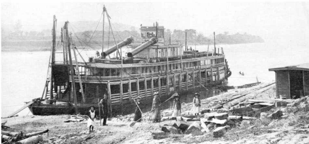
An unusual picture of the KATIE STOCKDALE taken at Harmar, O. (across the Muskingum from Marietta) in the Ohio River. Shown here in great clarity is how the smokestacks of old-time boats were lowered. An A-frame carried on the forward roof was used in the operation. When the stacks were down, each resting on a "yoke," the A-frame stood higher than the pilothouse. Then it had to be lowered to the roof. This picture shows it in the upright position. The virtue of this method was that the smokestacks, lowered, were completely out of the way. The accompanying story tells how the KATIE was taken under the K&M bridge at Point Pleasant by dismantling her pilothouse.
