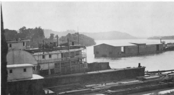
The 200-ft. Greene Line wharfboat built on two wooden pontoons each 20 ft. wide is being backed out of the Kanawha River in tow of the GREENDALE at the right. At left is the side-wheel GREENLAND on the docks. Picture was taken by C. C. Bowyer.
