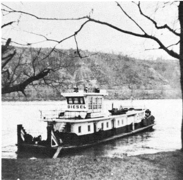
SAME BOAT as above in her commercial days, then named DIESEL. Built with a steel hull in 1926 by Dravo, she was first operated by Glyde Paden and J. C. Williamson. Then for a long period she was owned by M and O Dredging Co., and lastly by Seneca Towing Co. Gene Fitch bought her in 1967, put in a G-M 4-71 diesel, added a cabin behind the pilothouse, and gave her a luxury interior. Hull 90x16.
