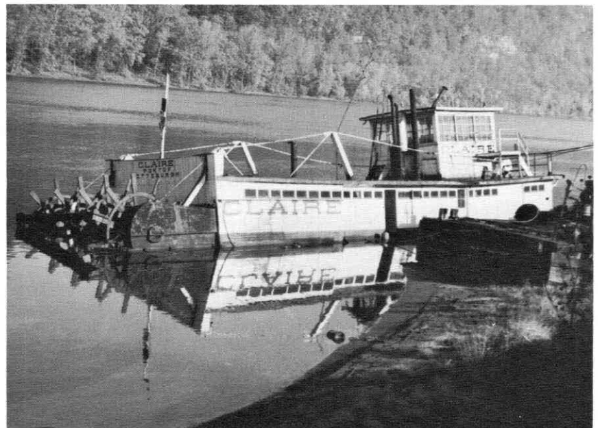
NO RELATION to the other two pictures on this page, the CLAIRE sank at Shippingport, Pa. on the Ohio last fall and was photographed on Oct. 18, 1969 by William E. Brandt of Steubenville. This wood hull sternwheeler was built in 1930, hull 79.7 x 18.8, operated most of her career by M and O Dredging Co.
