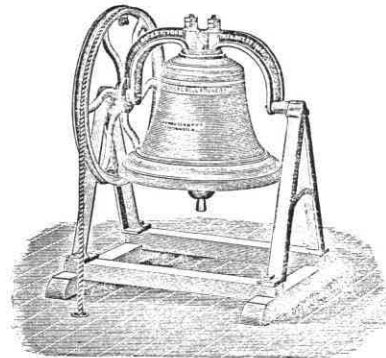
RANGING from 100 pounds to 350 pounds, mounted with our Improved Patent Rotary Hangings, by means of which the Bell can be readily turned in the Yoke, so as to present a new point for the stroke of the Clapper, when desired. Yoke, Frame of Ash timber, Iron Stands, and Iron Wheel.
