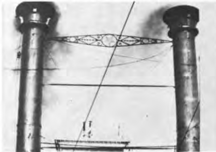
UPSIDE DOWN SPREADER on QUEEN CITY after extensive rebuilding and new smokestacks placed at Pt. Pleasant, W. Va. in 1913.
