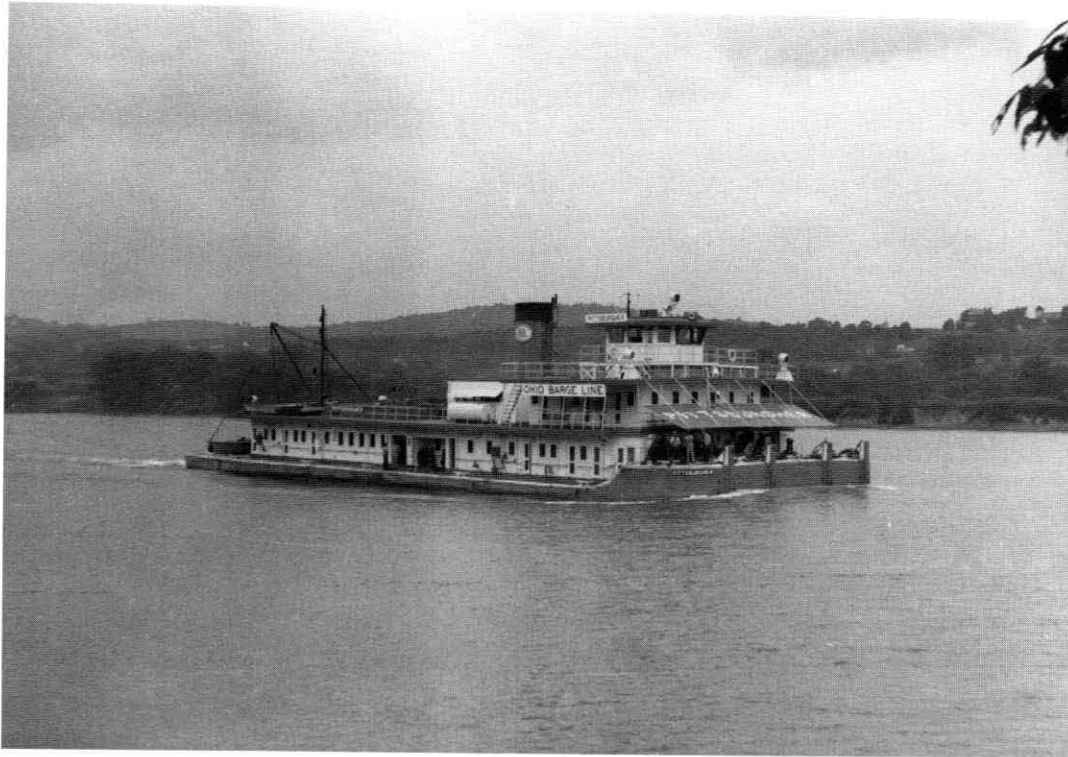
The twenty-one towboats built by the Defense Plant Corporation during World War II had a no-nonsense, muscular look even when not tied into a big tow of barges. This is the PITTSBURGER (T2059), built as the BOU ARADA and then called SOHIO FLEETWING before renamed by Ohio Barge Line in 1949. Photograph by William E. Reed.
